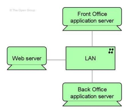
A device is a **specialization of a node** that represents a physical resource with processing capability.
