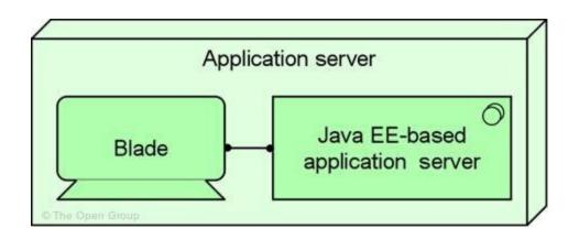
Nodes are active processing elements that execute and process artifacts, which are the representation of components and data objects.
