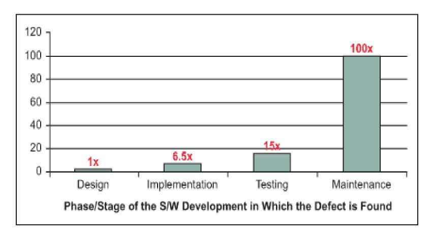
Cost of correcting an error in requirement specifications increases as we move through lifecycle phases
