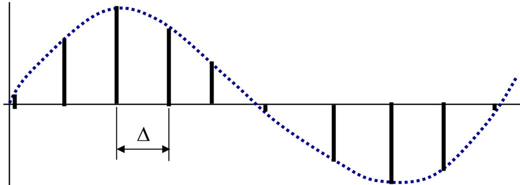
If the sampling interval  $\Delta$  is not at least half of the period of highest frequency  $F_{\max}$ , correct reconstruction is not possible
