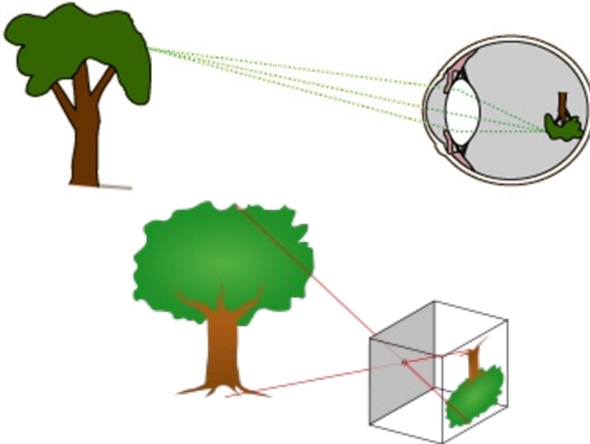
Pinhole camera - [http://en.wikipedia.org/wiki/Pinhole\\_camera](http://en.wikipedia.org/wiki/Pinhole_camera)
