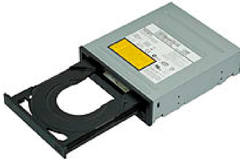
Compact discs, DVDs, and Blu-ray discs are common types of optical media which can be read and recorded by such drives
