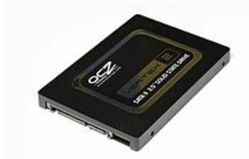
**SSD** has no moving parts and it only uses silicon as its media
